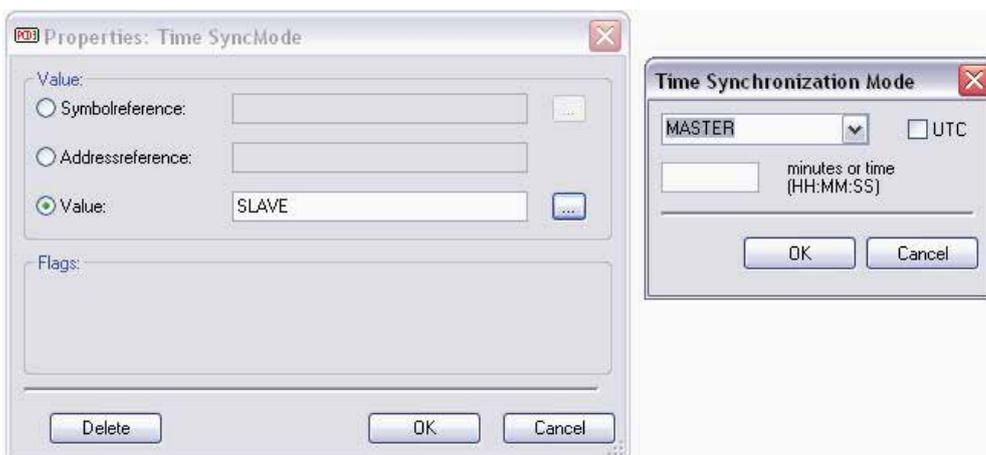
A Checkbox sets whether the synchronisation telegram will be set up as local time or as UTC.
