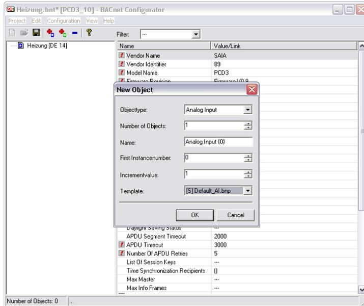
In „Standard View“ only a small part of the Properties are visible, all required properties will be parameterized with useful default values.
