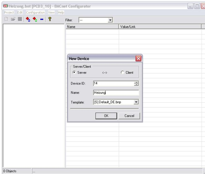
The (Slave) device object offers the possibility to Enable/Disable the complete communication to a specific server and to attach this to a PCD Flag. A register can also be attached to the communication status information.
