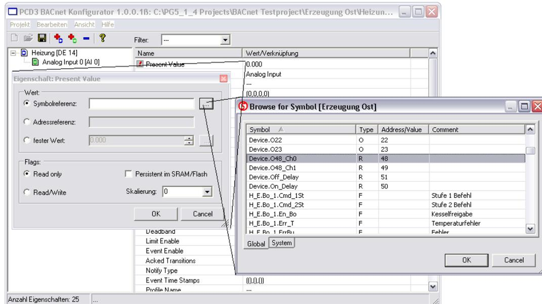
A Register for any real value with an selection of the conversion factor. Since the real value of BACnet is stored internally as an integer, a factor of 10 is necessary to store with an accuracy of tenth of the unit.
