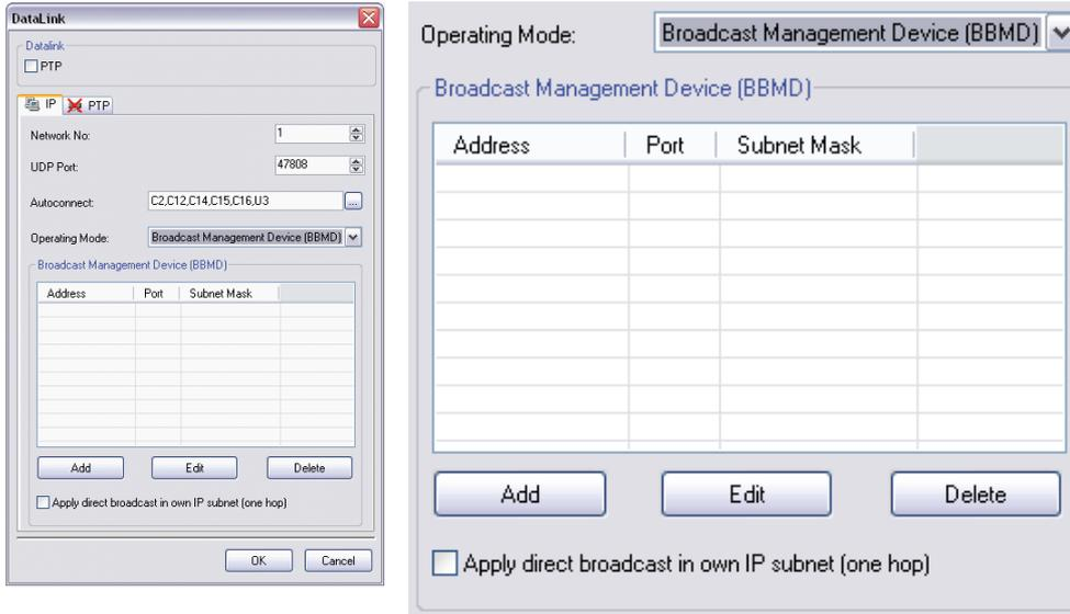
A list with the IP address of all other BBMD's in the network can be entered and on the bottom there's an option for using "One Hop" IP routers. Since those are not well spread, this option can be left unchecked in most applications.
