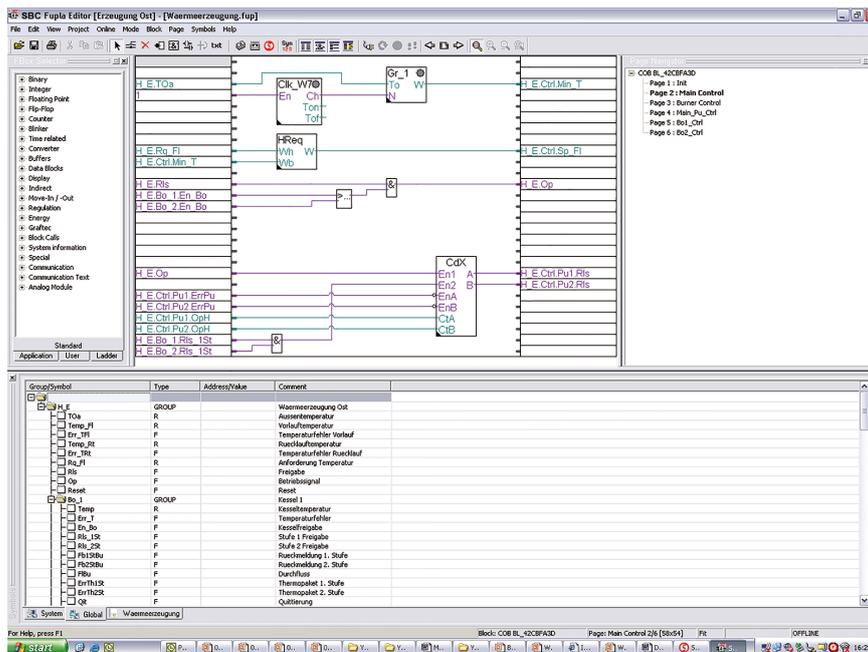
The usage of groups of symbols not only helps better structuring the data but also enables usage of Templates to faster create and parametrize objects. More details refer to Chapter 4.11.
