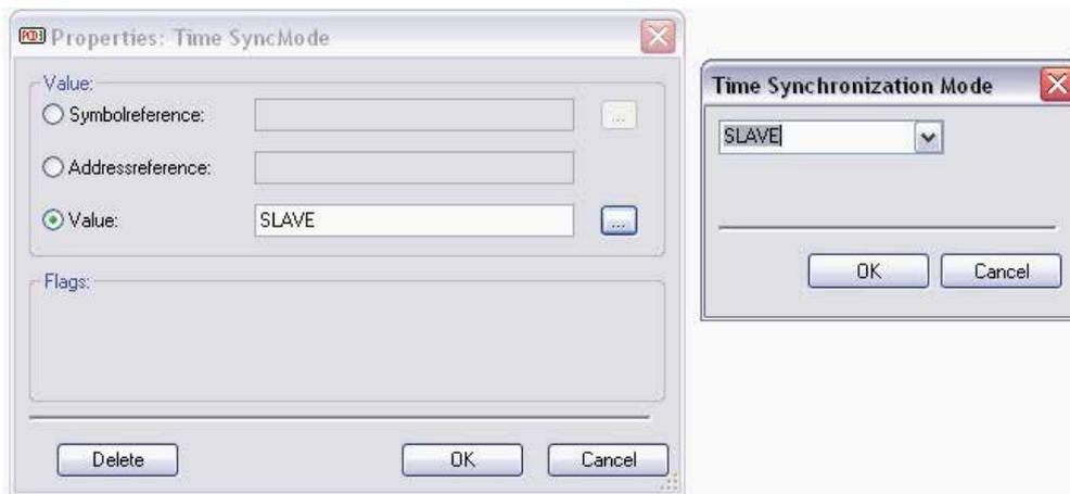
Only a one time synchronisation with the configuration PC using the Functionality in the "On-Line Configurator" in PG5 is required to activate the combined "Local Time"/"UTC Time" Real Time Clock.
