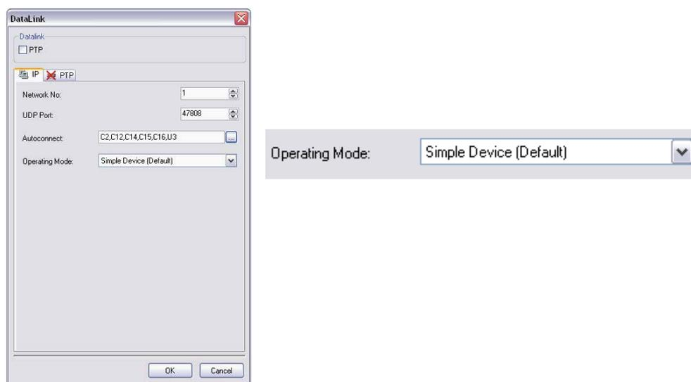
No parameters are available and no BBMD related functionality is activated on the PCD3 with this setting.
