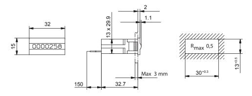
CMA152, with manual reset, flush mounting, mounting with tension spring
